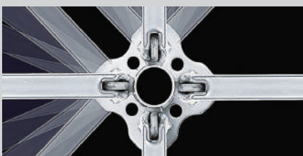
The rosett on the standard allows for connections up to 45°. The nodes at spacings of 50 cm also provide connection possibilities in all directions.
