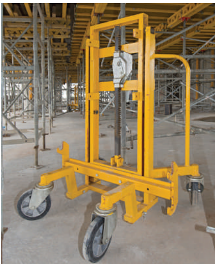
A trolley and winch facilitates the movement of PERI PD8 Tableform.
